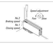
Two speed adjustment Closing Speed (150°  $\sim$  10°) Braking speed (10°  $\sim$  0°)
